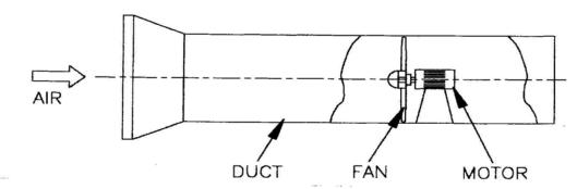
**Efficiency**: The measure of how well a fan does work against the total pressure to move a given volume of air is termed as Fan Total Efficiency. In general, a non – uniform air stream(flow) results in a less efficient fan. A fan equipped with a duct having proper inlet and outlet shapes, allows for a more uniform air stream (flow) and thus dramatically improves the efficiency of the fan; in fact, if properly designed, a ducted fan can achieve efficiencies up to 85%.
